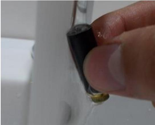
**Step 3:** After this, place your atomizer with its battery connection side UP on a piece of cloth or tissue and leave it out to dry overnight.
